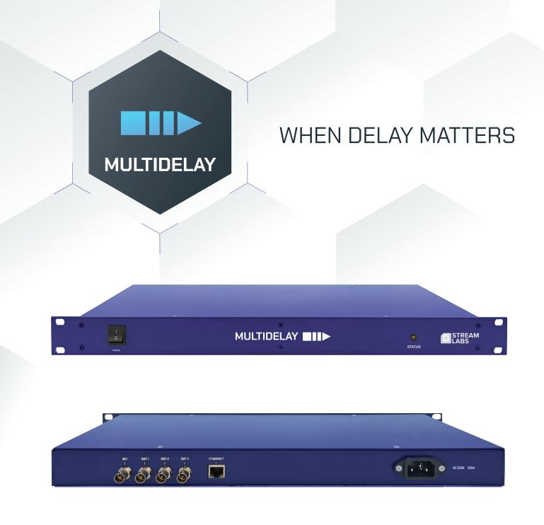
Stream MultiDelay is a hardware—based solution, which provides a delay of SD—SDI/DVB—ASI signal from 0,1 ms to 2 seconds, adjustable in a pitch of 0,1 ms and has a convenient management web—interface.
